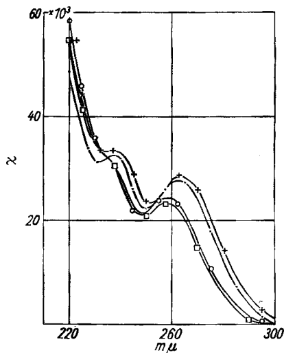
Abbild. 5. UV-Absorptions-Spektren von Diacetyl-dihydrophenazin (Ib) - - - -, Diacetyl-dihydro-1-methyl-phenazin (IIIb) □-□-□, Diacetyl-dihydro-1-acetoxymethyl-phenazin (IVb) ○-○-○, Diacetyl-dihydro-2-methyl-phenazin (XI b) +-+-+ (in 95-proz. Äthanol)
